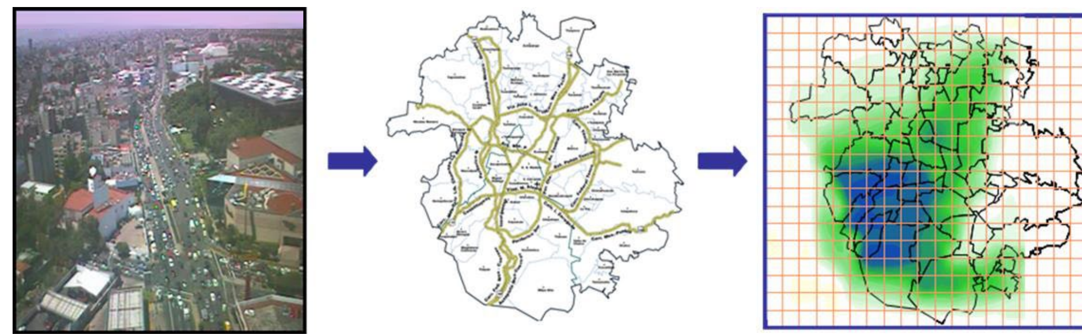
Figure 1. Emissions inventories are estimated by applying approximations and assumptions of the underlying physical and chemical processes in "real-world" emissions.
